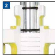
**2.** Safety gland packing made of PTFE silk; gland follower with double O-ring seal to prevent ingress of water into the packing area
