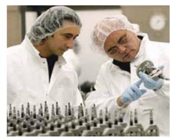
Our state of the art ISO 14644-1 compliant clean room is equipped with an ultrasonic cleaning system, featuring air locks for materials, and a test booth where leakage tests for strength and helium testing are conducted to determine the gas-leak tightness of the bellows and valve bodies. These tests are followed by vacuum compliant packing of the finished valves.
