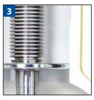
**3.** Protected multiple wall bellows made of 2.4819/Hastelloy C276, designed for 10.000 cycles, installed beyond main flow area
